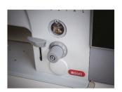
Stitch length adjustment knob (adjustable stitch length) up to 9mm
