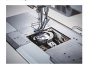
XXL (Super Large) Hook increases 70% of the bobbin thread volume and improves work efficiency
