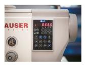
Integrated electronic control (direct drive motor)
