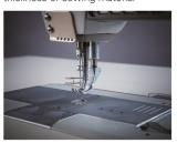
The presser foot lift can be raised up to 20mm
